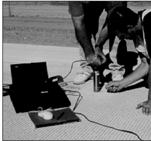
Figure 7. Typical impact-echo set-up for field applications.
