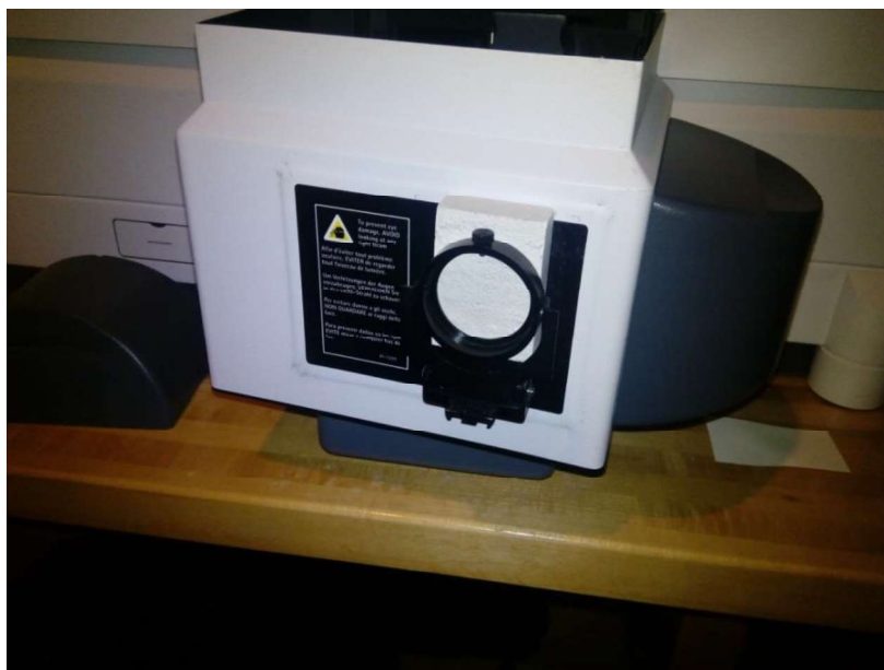
Figure 4. Testing of photocatalytic sample with UV-Vis-NIR Cary 5000 spectrophotometer.
