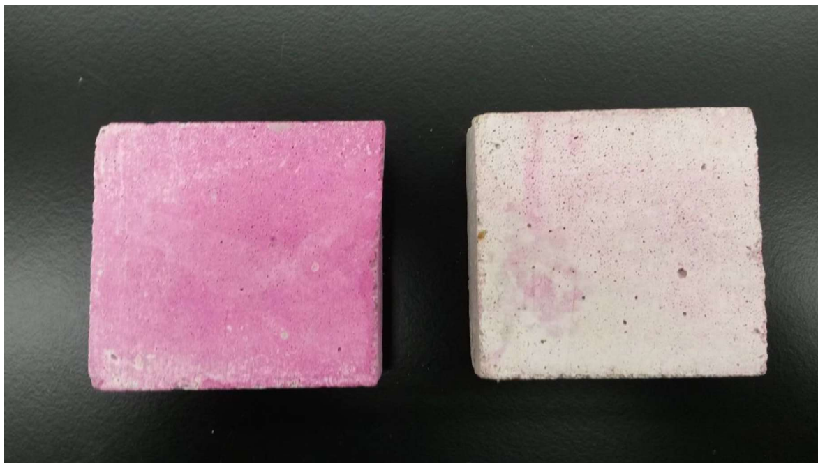
Figure 2. Side-by-side image of surfaces of non-carbonated (left) and carbonated (right) white TiO 2 , 0% fly ash mortar specimens after treatment with phenolphthalein.
