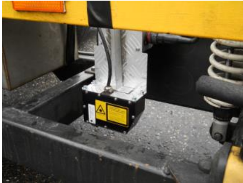
Figure 3: The laser texture meter mounted on the rolling resistance trailer in order to perform mobile measurements
