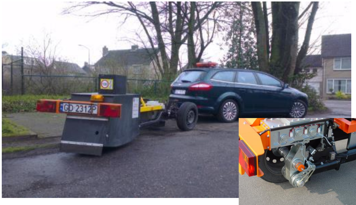
Figure 1: The TU Gdansk measurement trailer for measuring rolling resistance on road surfaces. The detailed photo provides a view of the measuring wheel over which a wind deflector is placed during measurement.
