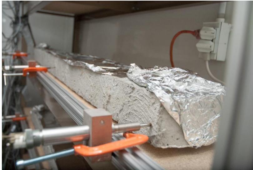
Figure 1. Beam curling setup with mounted LVDTs.
