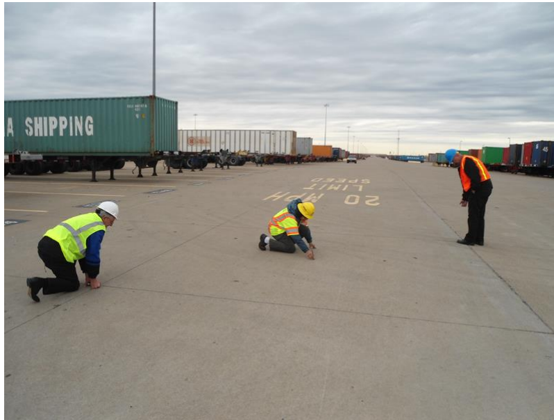
Figure 5. Curl measurement in the UP intermodal facility slabs
