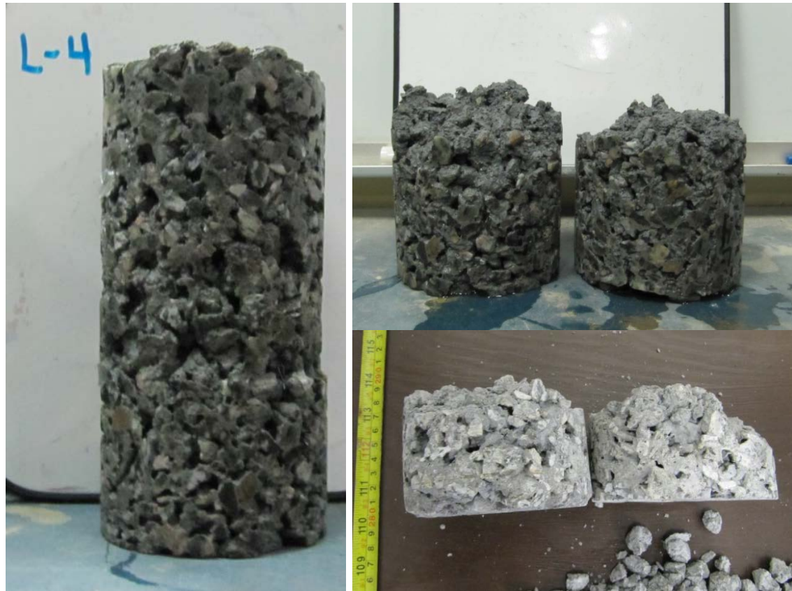
A. 69 cycles, B. Failure at 100 cycles, C. Remaining intact portion of core Figure 4: Failure of Latex Core (4)
