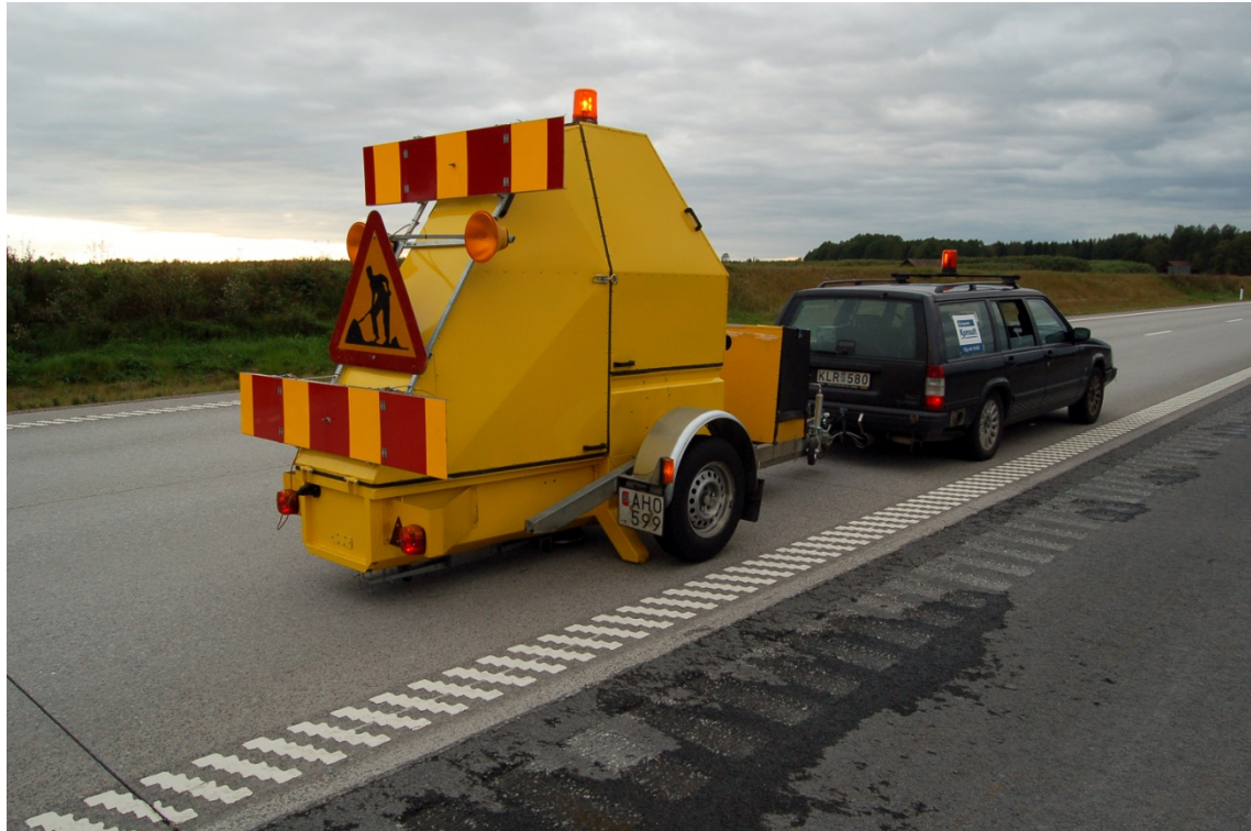
Figure 2. The FWD at the PCC test site on highway E4.
