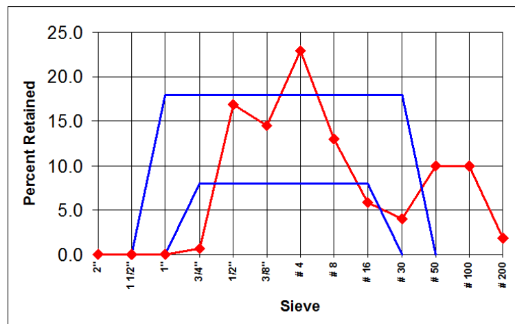
Figure 7. Haystack plot showing two low points at #16 and #30 sieves, indicating a high risk of segregation (Taylor, 2006). (1in=25.4mm)
