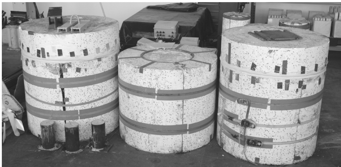
Figure 4. The polystyrene forms used during the tests of heat development in maturing concrete.
