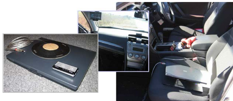
Figure 4 - Seat pad with USB link to laptop and wireless GPS receiver
