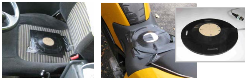
Figure 1 - Instrumented seat-pad for measurement of ride vibration
