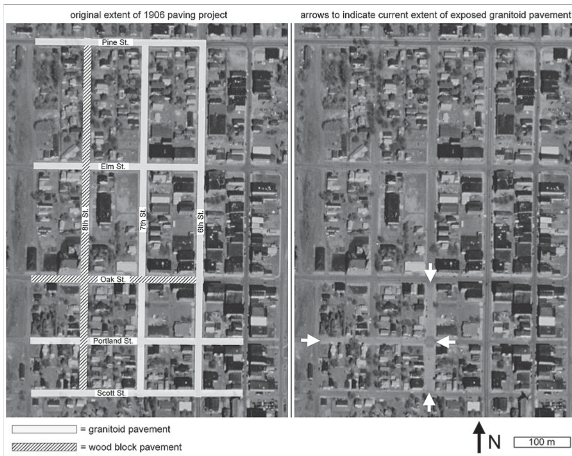
FIGURE 2: USGS aerial photography from 1998 showing extent of the 1906 street improvement project, (left) and white arrows to show present day extent of exposed granitoid pavement (right).
