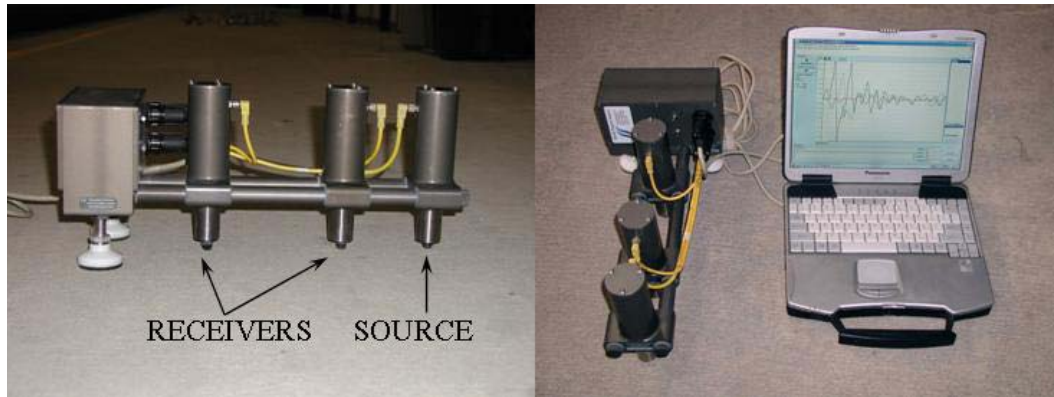
FIGURE 9. Portable Seismic Pavement Analyzer (PSPA)
