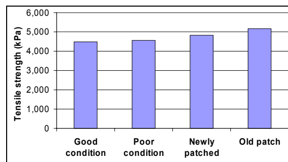
c) Compressive and Tensile Strength of Concrete Slabs
