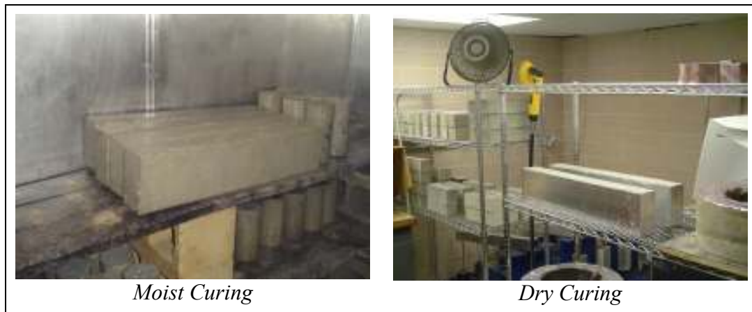
Figure 2. Moist and dry curing chambers.
