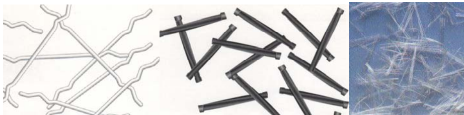
Figure 3 The fibres used in the Roermond pilot project. From left to right: long and short steel fibres and synthetic fibres.
