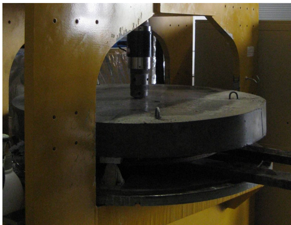
Figure 17 – The ASTM C1550 Test Rig (with test specimen)
