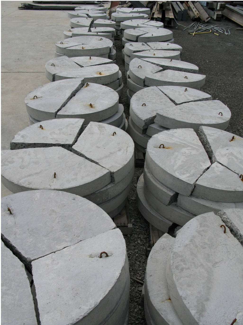
Figure 19 – ASTM C1550 panels after testing
