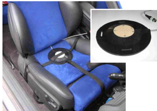
Figure 1 - Instrumented seat-pad for measurement of ride vibration.
