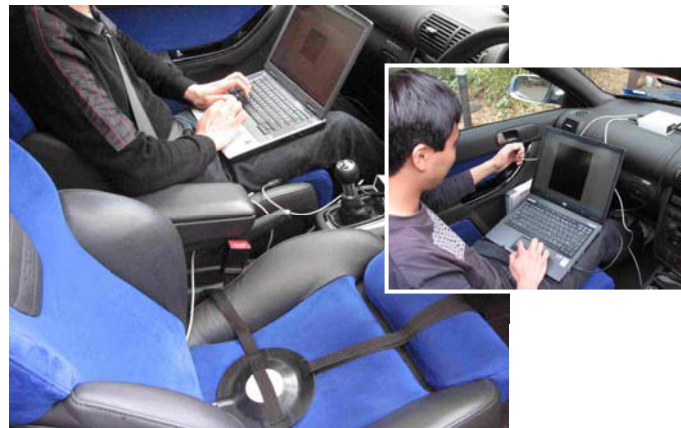
Figure 5 - Seat pad, laptop, USB-based DAQ and push button event marker.
