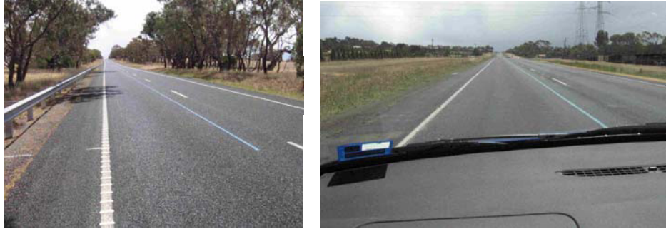
Figure 7 - General views of two test sections showing the blue line (left of the centre line) to aid tracking repeatability.
