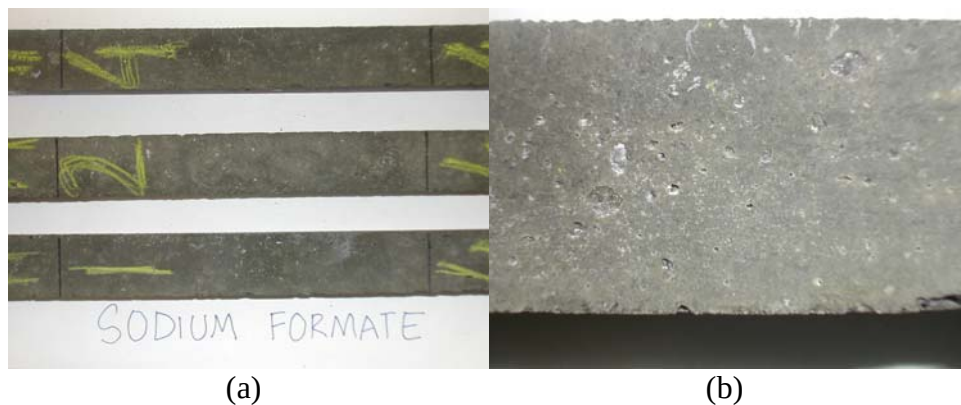
Figure 9. (a) Mortar bars containing Spratt aggregate soaked in saturated solution of sodium formate-based show no arching effect and (b) No evidence of distress on surface of mortar bars.
