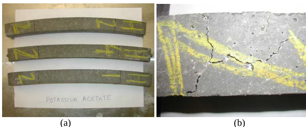
Figure 3. (a) Mortar bars soaked in 50% potassium acetate-based deicer soak solution showing development of arch and (b) Cracking on surface of mortar bars
