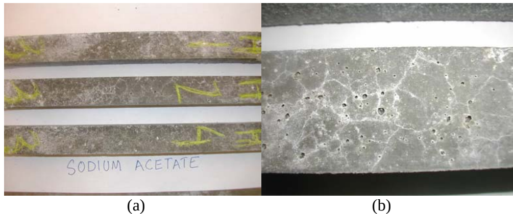
Figure 7. (a) Mortar bars soaked in saturated solution of sodium acetate-based deicer showing (no significant arching) and (b) Mild-cracking on surface of mortar bar
