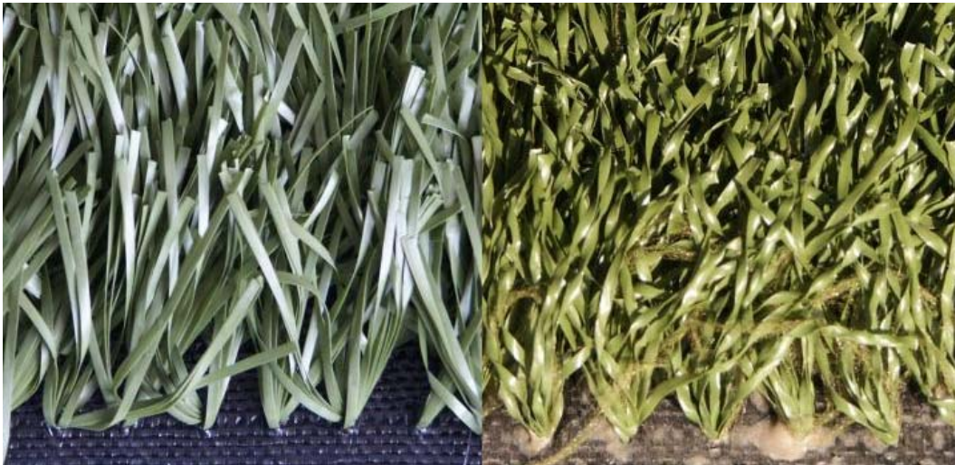
Figure 6. The type of artificial turf (especially the pile height and type of filaments) has to be matched to the concrete properties and placement conditions.
