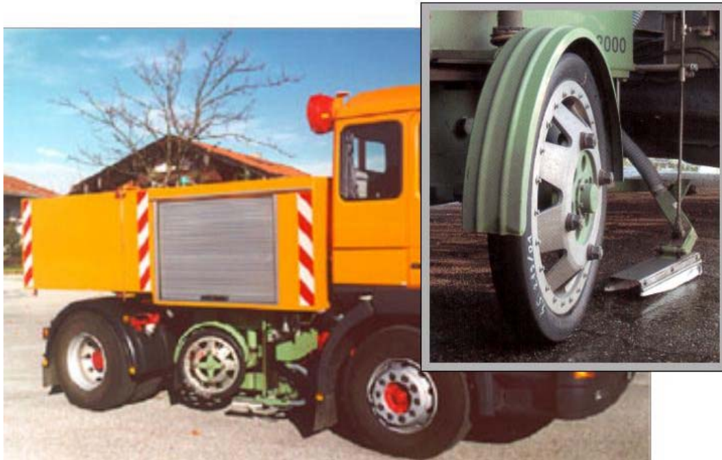
Figure 1. Sideway-force Coefficient Routine Investigation Machine (SCRIM), a high-speed measuring system used in Germany for measurement of the skid resistance of road surfaces.
