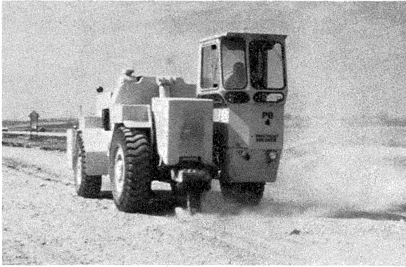
Figure 25. Backhoe equipment with rhinohorn removing steel from broken concrete on I-35 project in Iowa.
