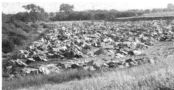
Figure 2. On I-80 in Nebraska the old concrete unsuitable for recycling was temporarily stored. Later recycled for use as riprap or shoulder maintenance material.
