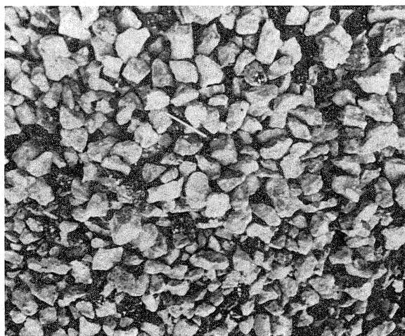
Figure 3. Recycled 3" coarse material used as subbase material on Eden's Expressway in Illinois.
