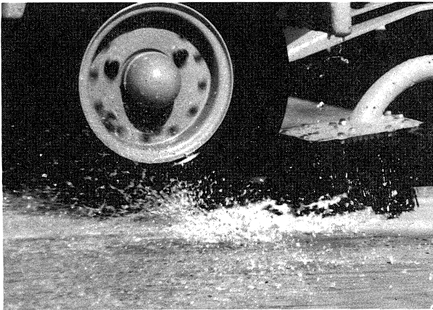
Figure 6. Self-watering system in operation.
