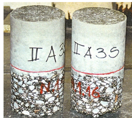
Shearing test on a concrete specimen on asphalt-treated granular material
