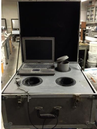
Figure 4. Calorimetry test device for heat of hydration of concrete (Taylor and Wang 2015)
