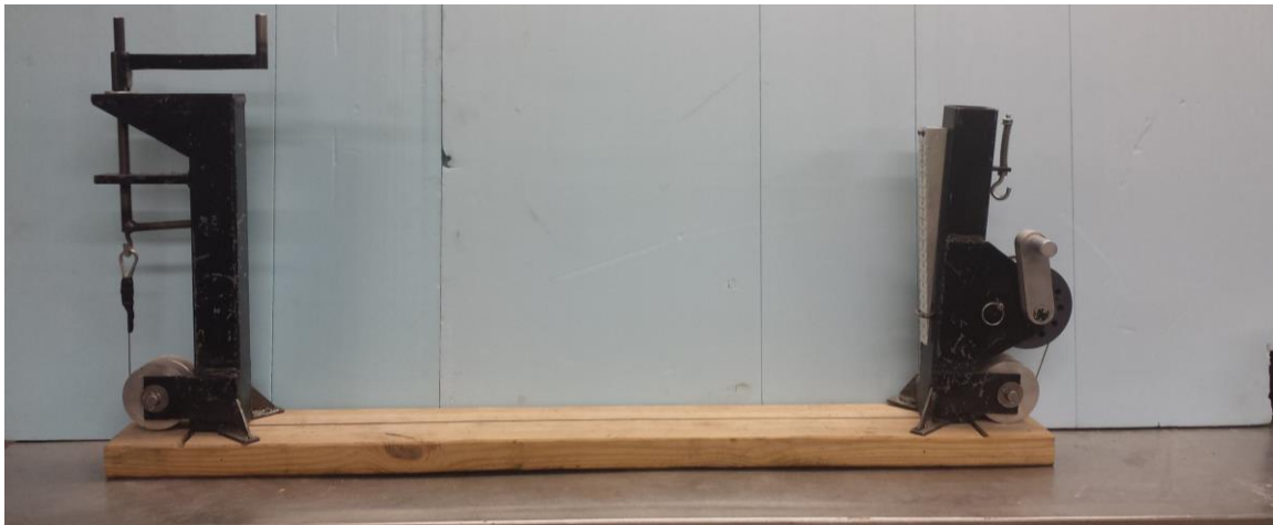
Figure 1. Overview of modified ISU curling and warping measurement device.
