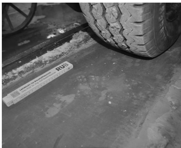
Figure 6. Early mechanical load: rolling tire on the surface of specimen B1 (first cycle)
