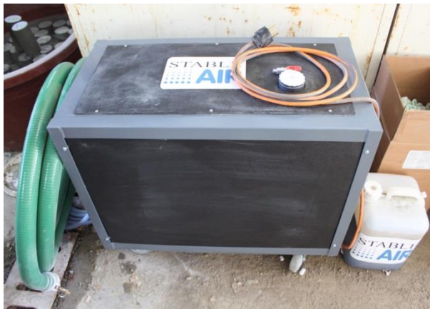
Figure 2.3(c) Foam generator
