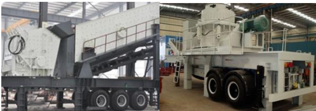
Figure 3: Mobile Impact Crusher Figure 4: Mobile Cone Crusher
