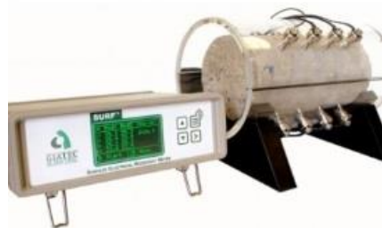
Figure 1: Device for Measurement of Surface Electrical Resistivity
