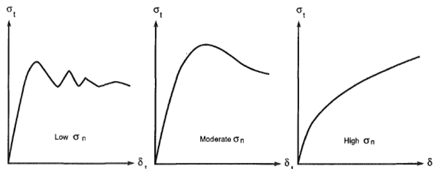
Figure 6 Shear stress vs. shear displacement at various level of constant normal stresses [29]
