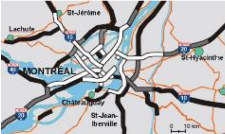
Figure 1 – The highway network in Montreal (Cormier & Thébeau, 2004). White sections = concrete pavements, black = asphalt.
