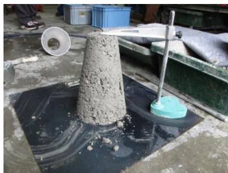
(a) low slump concrete (M-1)
