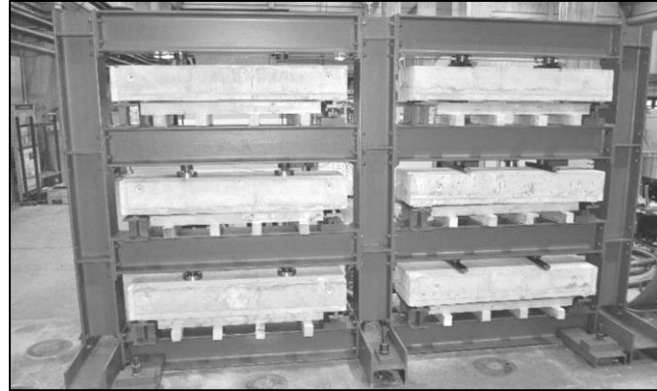
Figure 1. Test setup for simultaneous testing of six beams in a 4-point-flexural-test
