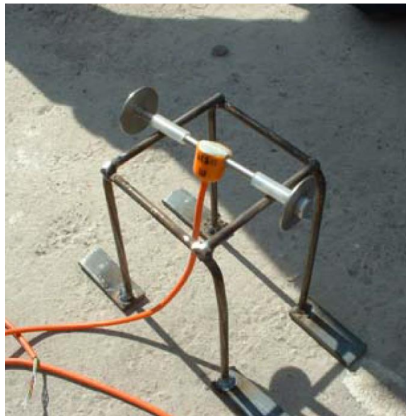
Figure 4. Typical vibrating wire strain gauge used.
