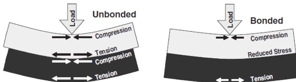
Figure 8. Comparison of theoretical unbonded and bonded overlay strain profiles (Rasmussen and Rozycki 2004).
