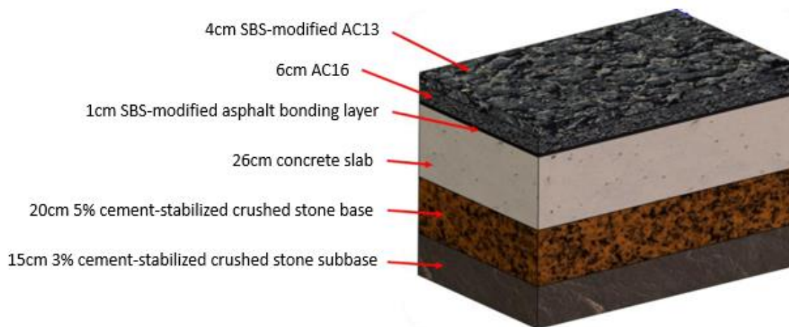
Figure 1. Zhejiang Test Section with HMA composite CRCP with BFRP bars.
