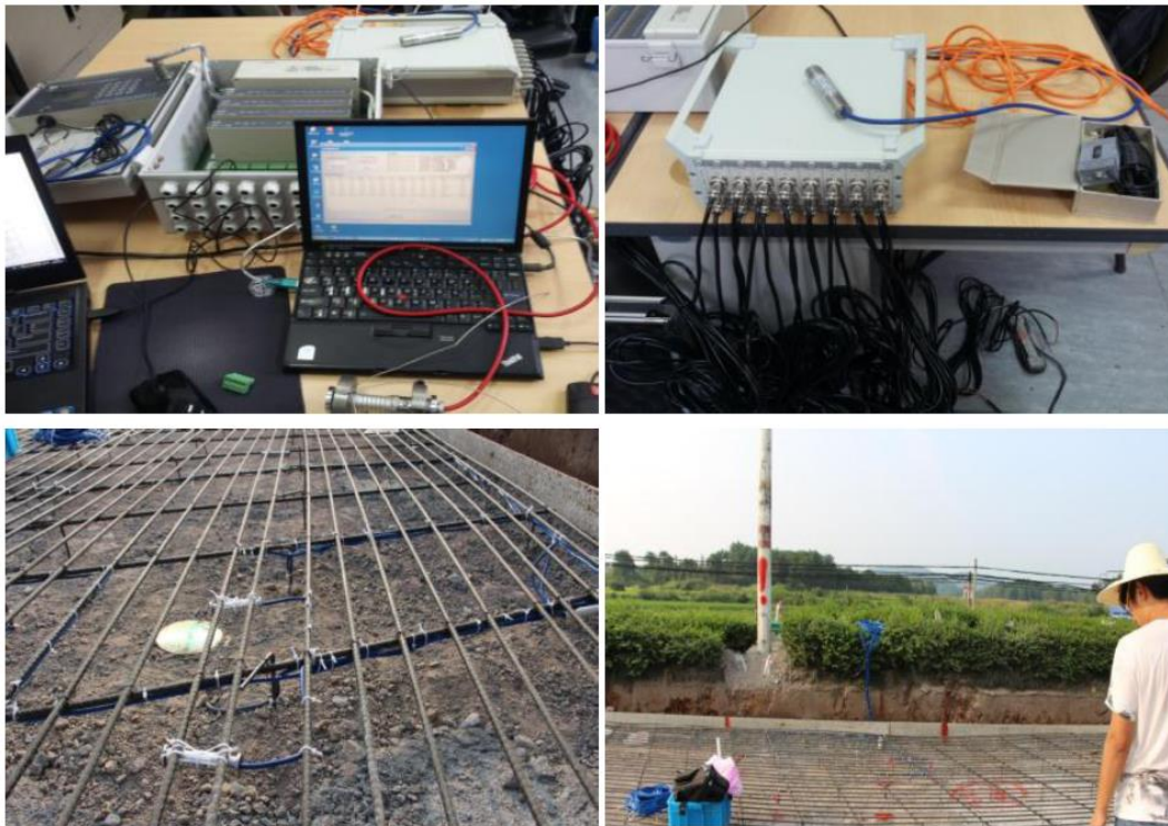
Figure 9. Data collection system and sensors in the CRCP layer.
