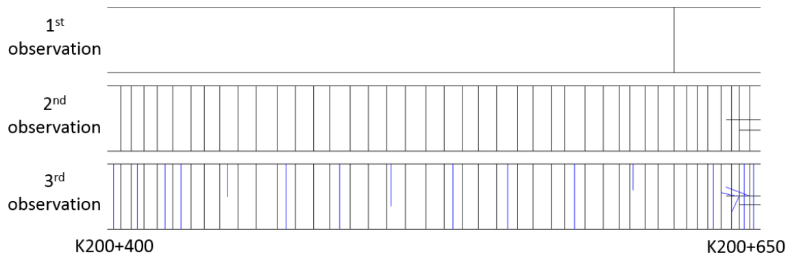
Figure 16. Crack maps of test section from observational surveys.
