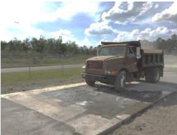
Figure 8. Load testing of the replacement slab using a 25,000 lb truck
