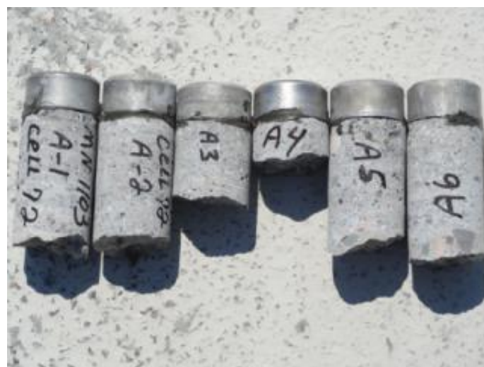
Figure 10. Fractured cores– cell 72 (left) and cell 71 (right).
