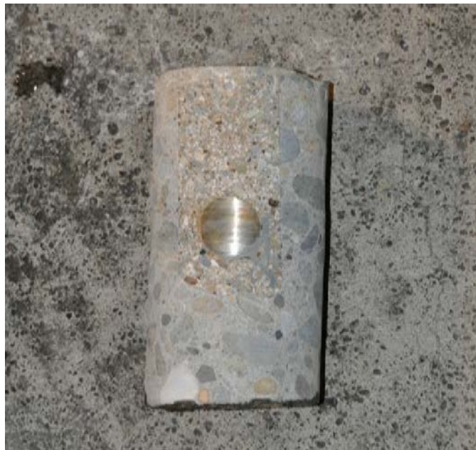
Figure 4. A core showing good consolidation from a DBR slot backfilled with polyester polymer concrete
