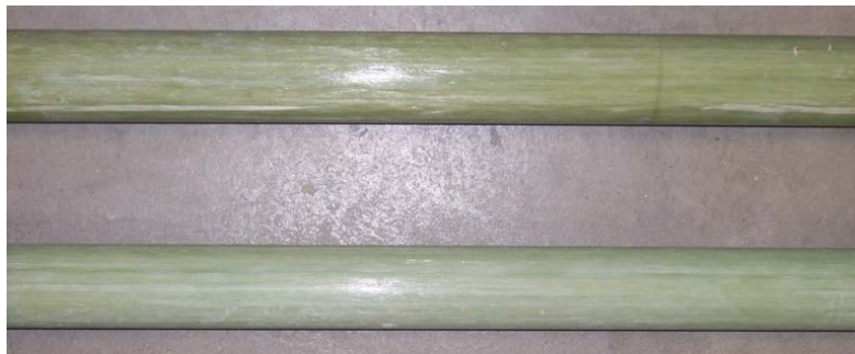
Figure 1: GFRP dowels of 34.9 and 38.1 mm-diameter
