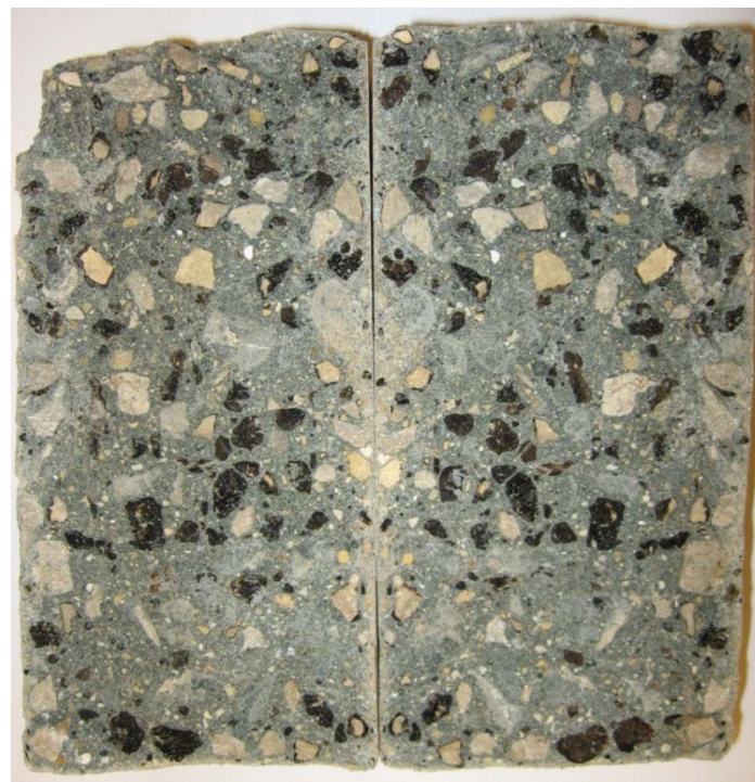
Figure 4. Split tensile specimen with 50% FRAP mix at 28 days. The bluish-turquoise color is due to slag hydration.
