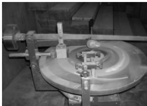
Figure 5. Abrasion Strength Testing Machine
