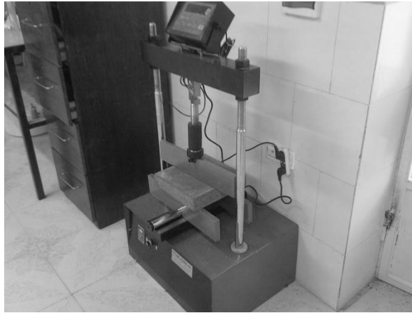
Figure 6. Flexural Strength Testing Machine
