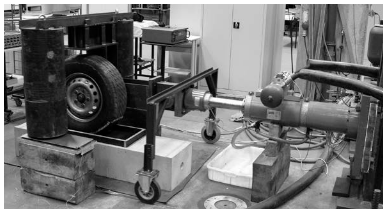
Figure 8. Penetration-test of sodium chloride solution due to over-rolling tire
