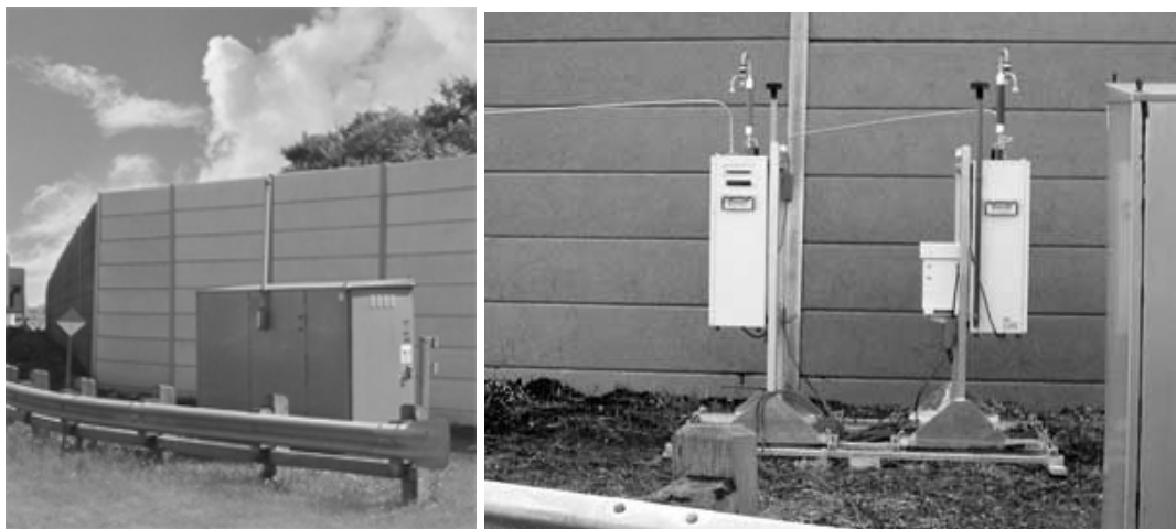
Figure 10: Photocatalytic concrete walls in Toronto (October 2011)
