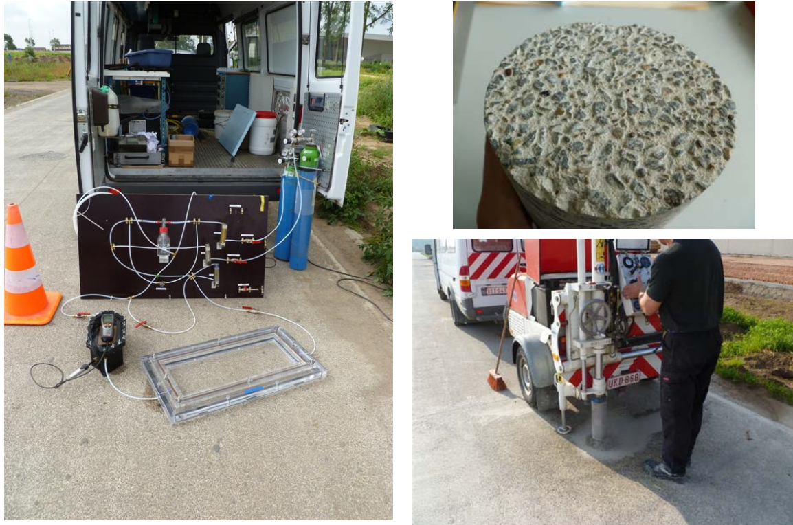
Figure 10 – Measurement of the photocatalytic efficiency on site and in the laboratory, on cores taken from the site.
