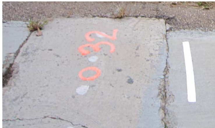
Figure 1. Test location marked with a circle to indicate location of the core hole and metallic tape spaced 61 cm away from the center of the core hole.
