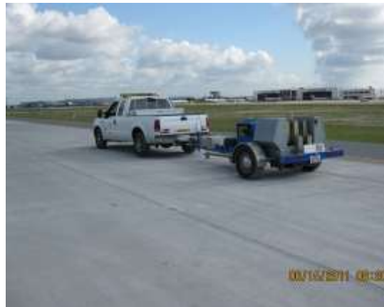
Figure 11 HWD and Load Plate.
