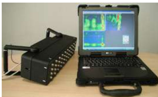
Figure 8a Ultrasonic Tomography ( www.pcte.com.au ) View of Sensors.
