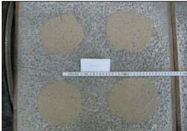
Figure 1 – Example of a test slab for texture measurements
