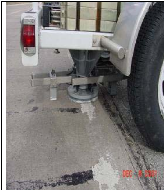
Figure 7-(a) Edge deflection measurement with asphalt shoulder
