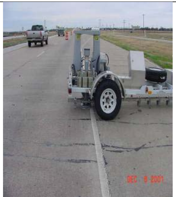
Figure 7-(b) Edge deflection measurement with tied concrete shoulder
