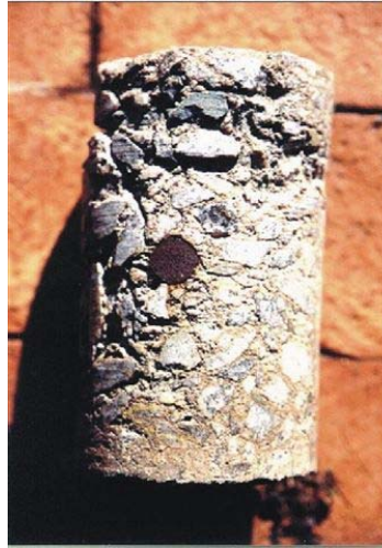
Photo 5: Weathering of concrete containing badly mixed cement/ggbs mixture, after 10 years' exposure to elements
