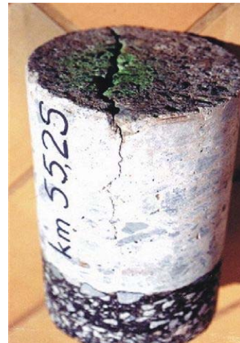
Photo 1: Surface weathering due to high ggbs content (left) Photo 2: Transverse crack showing no signs of pumping (right)
