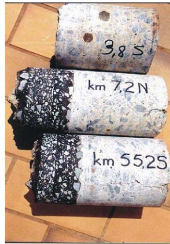
Photo 3: Intersection of transverse and random cracks (left) Photo 4: Good adhesion between asphalt and concrete (right)
