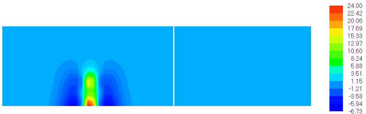
Figure 6. Graphical simulation of normal stresses (longitudinal direction on slab, position 3).
