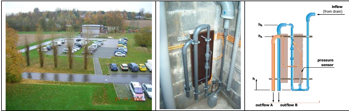
Figure 3 – Test parking lot and measuring device at the bottom of the structure
