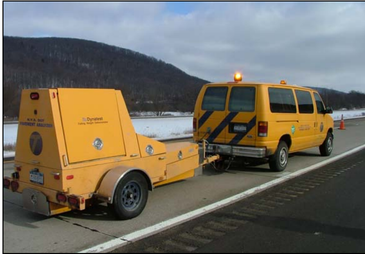
Figure 6 – Dynatest FWD device in March 2007
